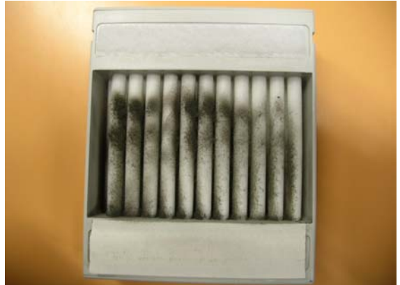
1) Dexwet filter after 4 weeks at work
